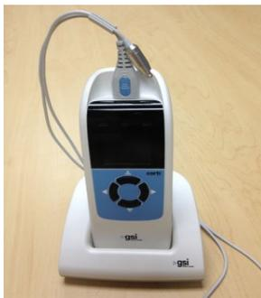
Make sure the probe holder is towards the end of the probe cable at the GSI wave logo / HDMI connector end. Gently push the probe cable into the probe holder at the point of the probe head.
