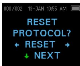
Selecting the ←RESET→ arrow key in the Reset Protocol menu will return the selected protocol settings to their original factory settings. Press the ↓NEXT key to exit.
