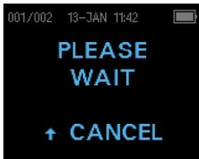
The Corti will search for the paired printer displaying 'Please Wait' while searching. When the printer is found, all test results stored in memory will print out automatically.
