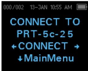
Printing to an optional thermal printer is by way of wireless connection. First establish wireless pairing between the Corti instrument and the printer by following the instructions in the section Instrument Settings - Wireless Device Pairing.
