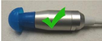
After selecting an eartip, push it onto the probe tube until it is flush against the base of the probe tube. Twisting the eartip slightly while pushing it onto the probe tube is recommended. Be sure the eartip is fully seated on the probe. There should be no gaps between the eartip and the collar of the probe head.
