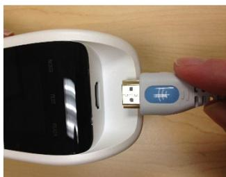
Insert the Probe's HDMI connector firmly into the socket on the top of the Corti. The plug will fit in only one direction. The GSI wave logo will align with the instrument control panel.
