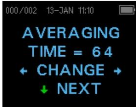
The *maximum* Averaging Time has four available settings. The Averaging Time sets the maximum test time to obtain a Pass and will affect the signal-to-noise ratio (SNR). For example, a setting of 32 seconds would stop the TE test after 32 seconds if the Pass criteria are not met.
