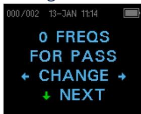
The number of frequencies for determining a PASS can be set from 0 to 6. **If the setting is on 0, then no indication of PASS/REFER will be made.** This setting is used in conjunction with the PASS SNR to set the criteria for the overall test PASS/REFER indication. For example, if the PASS SNR is set to 4 dB and the number of frequencies for PASS is set to 3 then the test must contain at least 3 frequencies where the emission is at least 4 dB above the noise to indicate a PASS.
